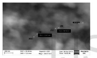
From the above SEM images we can infer that the as synthesized  ${\rm SnO_2}$  nanostructures exhibit crystalline morphology, particles are agglomerated and are non-porous.
